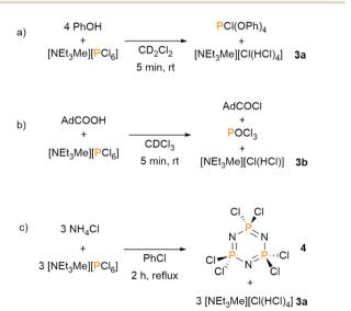
Scheme 3 [NEt<sub>3</sub>Me][PCl<sub>6</sub>] as a synthon for important reactions of PCl<sub>5</sub>. Ad = adamantyl.
