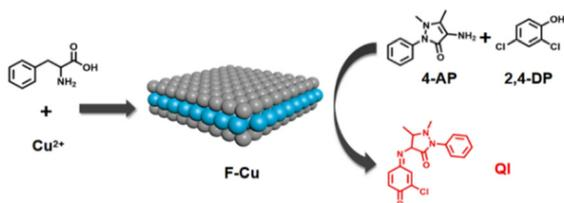
Scheme 1 Principle of colorimetric detection with F-Cu nanozymes.
