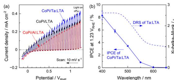
Fig. 3 (a) Current–potential curves obtained using CoPi-modified LTA, 5%Al-doped LTA and 5%Ta-doped LTA in aqueous 0.5 M Na<sub>2</sub>SO<sub>4</sub> solutions under simulated sunlight. (b) The IPCE spectrum for the CoPi/Ta:LTA photoanode at an applied potential of 1.23 V<sub>RHE</sub> together with the DR spectrum of the Ta:LTA particles.
