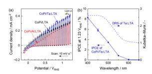
Fig. 3 (a) Current–potential curves obtained using CoPi-modified LTA, 5%Al-doped LTA and 5%Ta-doped LTA in aqueous 0.5 M  $\rm Na_2SO_4$  solutions under simulated sunlight. (b) The IPCE spectrum for the CoPi/Ta:LTA photoanode at an applied potential of 1.23  $\rm V_{RHE}$  together with the DR spectrum of the Ta:LTA particles.
