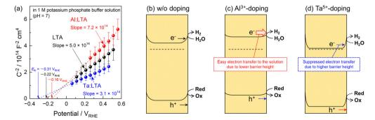
Fig. 4 (a) Mott–Schottky plots obtained from the LTA, 5%Al-doped LTA and 5%Ta-doped LTA photoanodes by applying a potential frequency of 5 kHz in a potassium phosphate buffer electrolyte under dark conditions. Schematic band diagrams for the (b) undoped, (c) Al<sup>3+</sup>-doped and (d) Ta<sup>5+</sup>-doped LTA samples at equilibrium in the aqueous solution under dark conditions, demonstrating the effects of aliovalent doping.
