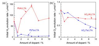
Fig. 2 Initial photocatalysis rates as functions of doping level as determined for the (a) hydrogen evolution and (b) oxygen evolution half-reactions under illumination with a 300 W Xe lamp ( $\lambda$  = 420–800 nm).
