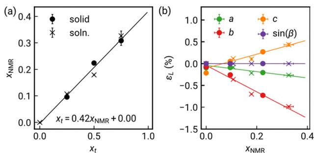
Fig. 2 (a) Determination of  $x$  through integration of solution  $^1\text{H}$  NMR spectra. Linear fit shown. (b) Variation in lattice parameter strain ( $\epsilon_L$ ) with linear fit. Data point for  $x_{\text{NMR}} = 0.31$  solid-state excluded due to presence of  $\text{NiCl}_2 \cdot 6\text{H}_2\text{O}$  impurity. Circles indicate solid-state samples, crosses solution samples.
