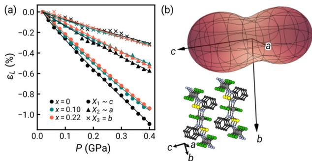
Fig. 3 (a) Linear strain ( $\epsilon_L$ ) along each principal axis determined through HP-PXRD for solid-state  $\text{NiCl}_2(\text{btd})_{1-x}(\text{bod})_x$ , with compressibility fit by an empirical equation of state.<sup>24</sup> (b) Linear compressibility indicatrix at  $P = 0.2$  GPa for  $x = 0.22$  (solid) with crystal structure in similar orientation.
