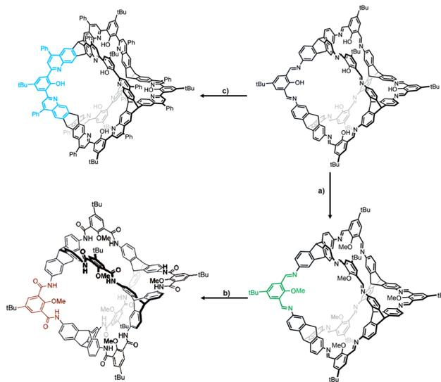
Fig. 6 Synthesis of stable POCs. (a) CH<sub>3</sub>I, K<sub>2</sub>CO<sub>3</sub>, DMF, 80 °C, 16 h; (b) NaClO<sub>2</sub>, NaH<sub>2</sub>PO<sub>4</sub>, 2-methyl-2-butene, THF, H<sub>2</sub>O, rt, 16 h; (c) Sc(OTf)<sub>3</sub>, chloranil, phenylacetylene (neat), 100 °C, 20 h.
