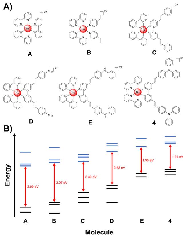
**Fig. 1** DFT-guided rational design of Ru(II) polypyridine complexes with absorption at longer wavelengths. (A) Proposed structures of metal complexes. (B) Computed frontier orbital energies and HOMO–LUMO gaps of proposed structures. Occupied orbitals are represented as black lines and unoccupied orbitals are represented as blue lines. The HOMO–LUMO gap is represented as a red arrow.
