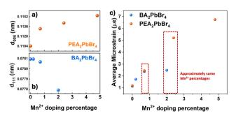
Fig. 2 The change in d-spacing against Mn<sup>2+</sup> concentration of (a) the (005) plane in PEA<sub>2</sub>PbBr<sub>4</sub> (b) the (111) plane in BA<sub>2</sub>PbBr<sub>4</sub> and (c) microstrain vs. Mn<sup>2+</sup> doping percentage.
