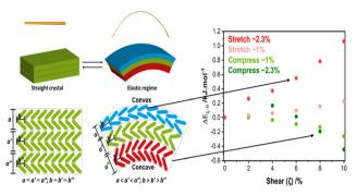
Fig. 3 Mechanical bending causes FMPES through uniaxial strain. Bending causes uniaxial tension (stretching) on the convex surface, and uniaxial compression on the concave surface. The latter reduces energy barriers needed for subsequent plastic deformation and the onset of mechanical activation. Figure adapted from ref. 59 with permission from the Royal Society of Chemistry.
