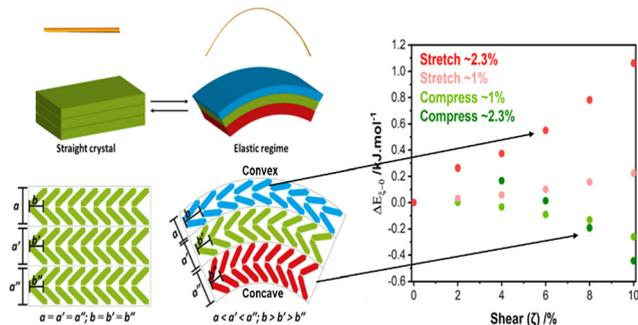
**Fig. 3** Mechanical bending causes FMPES through uniaxial strain. Bending causes uniaxial tension (stretching) on the convex surface, and uniaxial compression on the concave surface. The latter reduces energy barriers needed for subsequent plastic deformation and the onset of mechanical activation. Figure adapted from ref. 59 with permission from the Royal Society of Chemistry.
