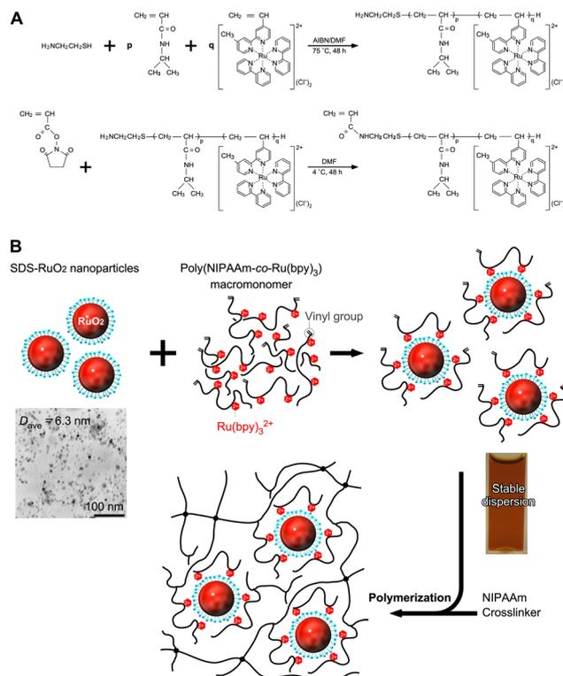
**Fig. 3** (A) Synthetic procedure for the poly(NIPAAm-co-Ru(bpy) $_3$ ) (PNR) macromonomer using telomerization and amide condensation. (B) Synthetic procedure for the PNR-grafted PNIPAAm gel containing  $RuO_2$  NPs by radical copolymerization using a crosslinker. Reproduced from ref. 67 with permission from Wiley-VCH, Copyright 2010.
