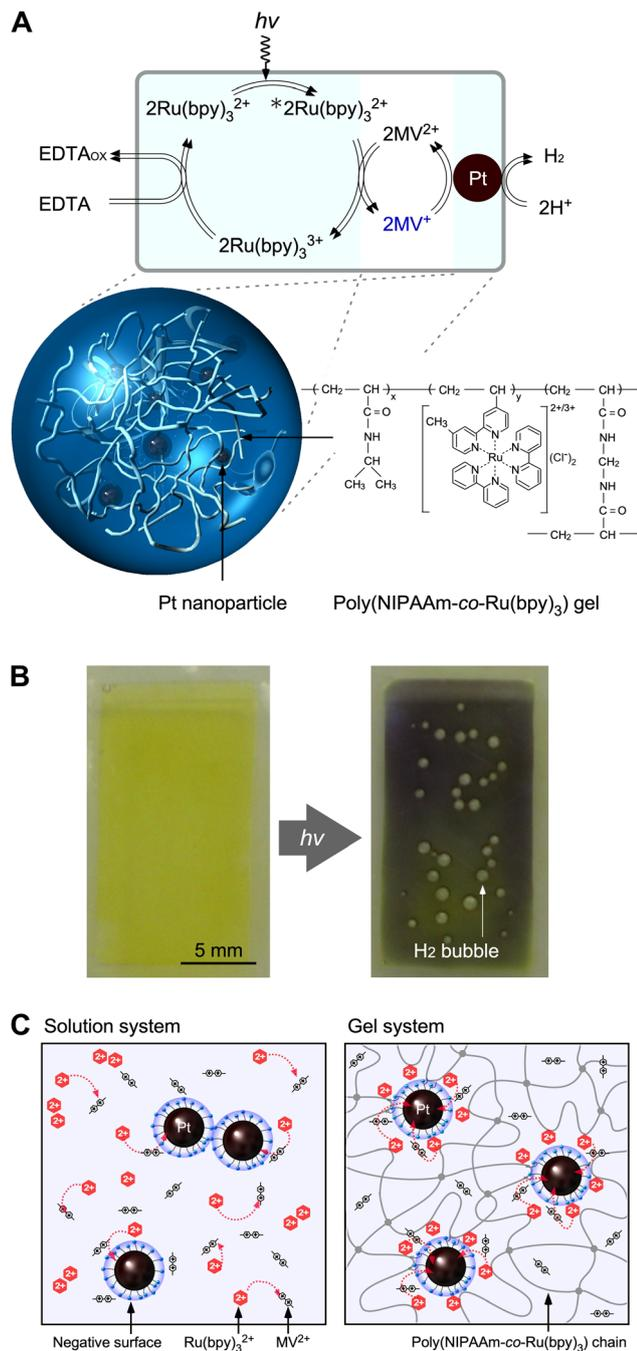
**Fig. 4** (A) Photoinduced H<sub>2</sub>-generating system using PNR gel containing Pt NPs. (B) Color change and H<sub>2</sub> bubble generation in the gel system under visible-light irradiation. (C) Schematic illustration of electron transfer in conventional solution and gel systems. Reproduced from ref. 68 and 69 with permission from the Royal Society of Chemistry, Copyright 2009.
