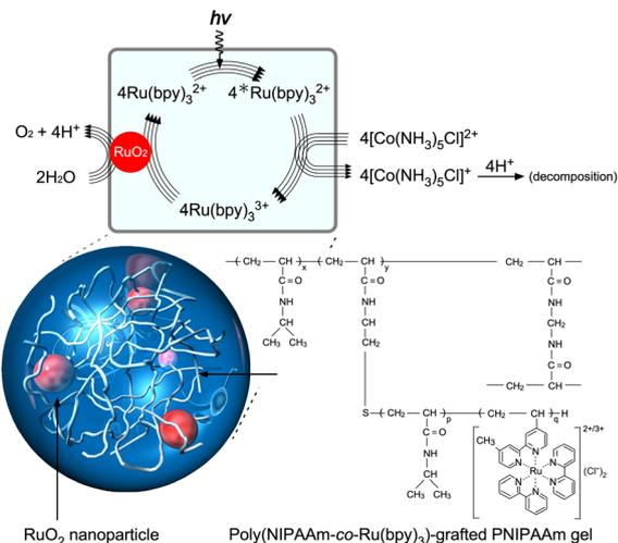
**Fig. 2** Photoinduced  $O_2$ -generating system using a poly(NIPAAm-co-Ru(bpy) $_3$ )-grafted PNIPAAm gel containing  $RuO_2$  nanoparticles (NPs). Reproduced from ref. 67 with permission from Wiley-VCH, Copyright 2010.
