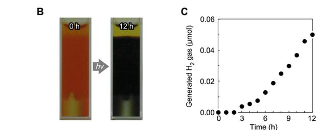
**Fig. 8** (A) Photoinduced H<sub>2</sub>-generating system composed of a poly(NIPAAm-*co*-Ru(bpy)<sub>3</sub>-*co*-viologen) gel containing Pt NPs. (B) Images of the gel suspension before and after light irradiation. (C) H<sub>2</sub>-generation in the gel system. Reproduced from ref. 68 with permission from the Royal Society of Chemistry, Copyright 2009.
