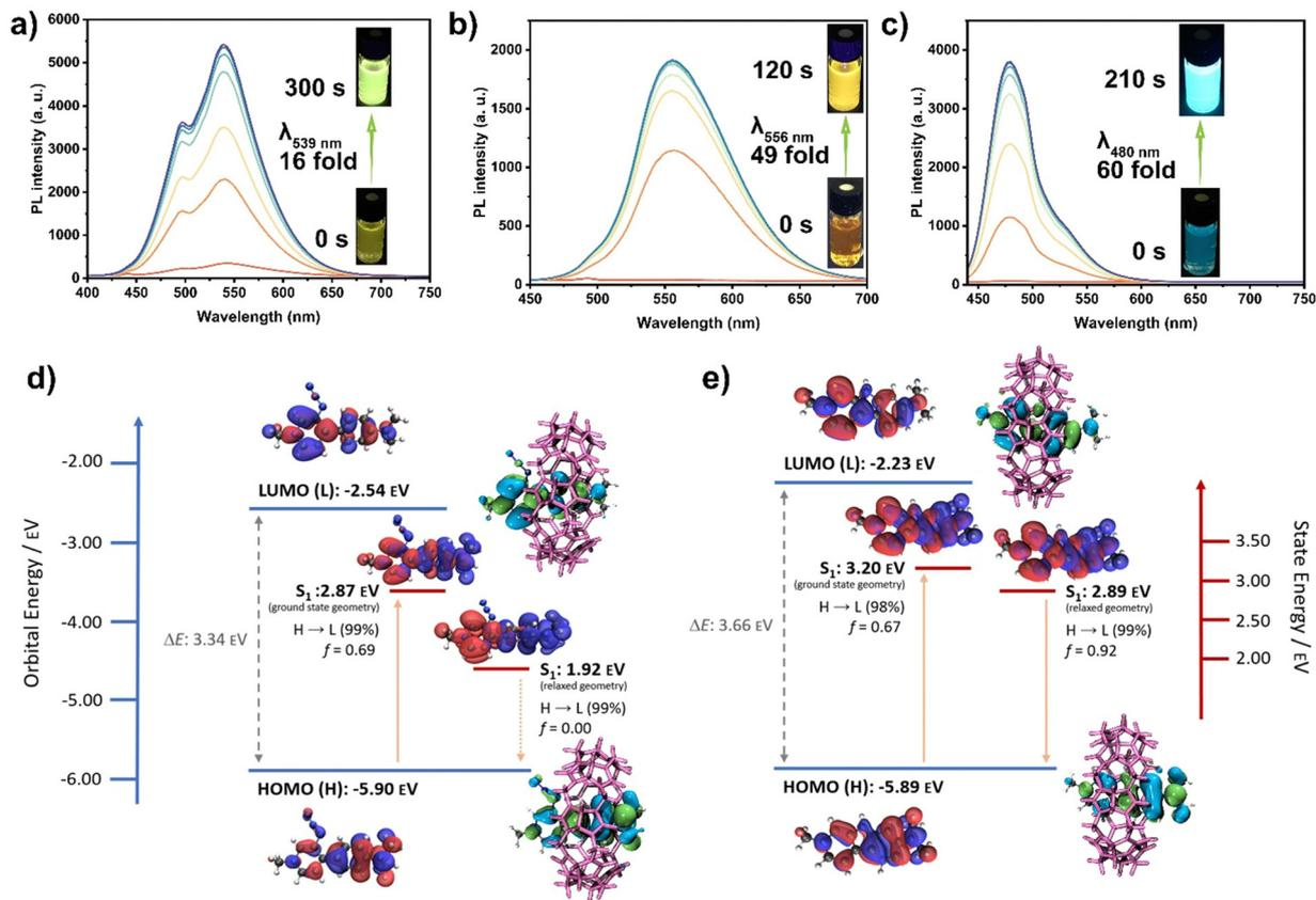
Fig. 2 Photoluminescence (PL) spectra of photolysis of (a) **Az-1**-CB7; (b) **Az-2**-CB7; and (c) **Az-3**-CB7 after different reaction times; (d) and (e) computed molecular orbitals (HOMO/LUMO) and difference density plots of the first excited singlet state at the ground state and relaxed  $S_1$  geometry of **Az-3** and **Cb-3**, calculated at the (TD-)DFT PBE0/6-31+G(d,p)//B3LYP/6-31G(d) level of theory in water (PCM).
