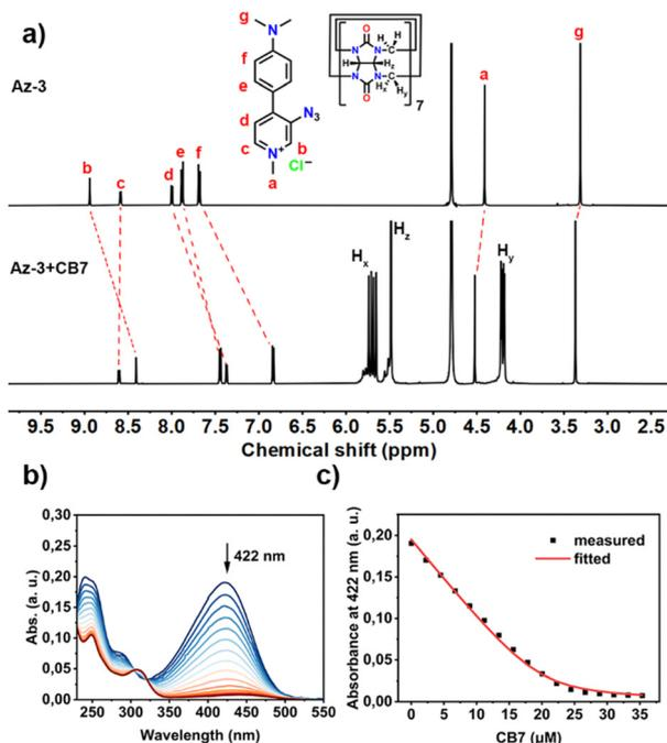
Fig. 1 (a) <sup>1</sup>H NMR spectra (500 MHz, D<sub>2</sub>O) of **Az-3** (0.5 mM) and **Az-3** + CB7 (0.5 mM each); (b) UV-vis titration spectra of **Az-3** (20 μM) upon addition of CB7 (0–35 μM) in water at 298 K, and (c) the binding isotherm fitted with a 1:1 host-guest binding model.
