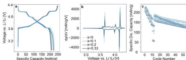
**Fig. 3** (a) First-cycle charge–discharge curves of LIB half-cells using LRLNO 0–750, 0.1–750, 0.2–750, or 0.33–750 at 25 °C and at 0.05C. (b) Respective second-cycle differential capacity curves. (c) C-rate testing at 0.05C, 0.1C, 0.33C, 1C, 2C, and 5C (two cycles each) followed by cycling at 0.33C. The error bars represent the standard deviation from three independent cells.
