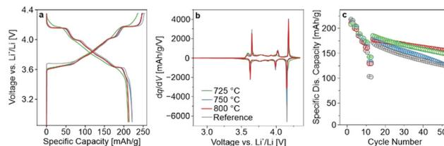
**Fig. 2** (a) First-cycle charge–discharge curves of LIB half-cells using LRLNO 0.2–725, 0.2–750, 0.2–800, or reference LNO at 25 °C and at 0.05C. (b) Respective second-cycle differential capacity curves. (c) C-rate testing at 0.05C, 0.1C, 0.33C, 1C, 2C, and 5C (two cycles each) followed by cycling at 0.33C. The error bars represent the standard deviation from three independent cells.
