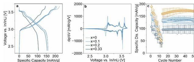
**Fig. 4** (a) First-cycle charge–discharge curves of SSB cells using LRLNO 0–750, 0.1–750, 0.2–750, or 0.33–750 at 45 °C and at 0.1C. (b) Respective second-cycle differential capacity curves. (c) C-rate testing at 0.1C (one cycle), 0.2C, 0.5C, 1C, and 2C (three cycles each) followed by cycling at 0.2C. The orange data points display the performance of LNO with a cobalt-based coating. The error bars represent the standard deviation from three independent cells.
