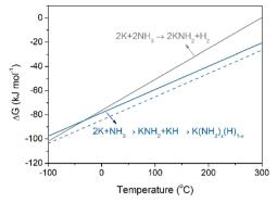
Fig. 3 Temperature dependences of  $\Delta G$  for reactions of K and NH<sub>3</sub> to form different products. The enthalpies of KH and KNH<sub>2</sub> are taken from the literature. <sup>15</sup> The entropies of solids are not considered. The dashed line serves as a guide, illustrating that the formation of K(NH<sub>2</sub>)<sub>x</sub>(H)<sub>1-x</sub> solid solution is thermodynamically more favorable.
