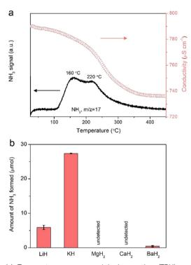
Fig. 2 (a) Temperature-programmed hydrogenation (TPH) profiles of  $NH_3$  signal (m/z = 17) and conductivity decrease during the hydrogenation of the nitrogen plasma-treated KH sample. Sample mass is 30 mg.  $P_{\rm H_2}$  is 1 bar. H<sub>2</sub> flow rate is 30 mL min<sup>-1</sup>. (b) The amounts of fixed N in metal hydrides determined through TPH measurements. Voltage is 12 kV. Sample mass for LiH is 10 mg, and the others are 30 mg.
