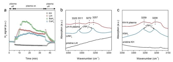
Fig. 1 (a) Time courses of  $H_2$  MS signals (m/z = 2) for LiH, KH, CaH<sub>2</sub>, and BaH<sub>2</sub> under nitrogen plasma. Voltage is 12 kV. Plasma power is ca. 8 W. FTIR spectra of LiH (b) and KH (c) collected after nitrogen plasma treatment and reference LiH, KH, LiNH2, and KNH2 samples.
