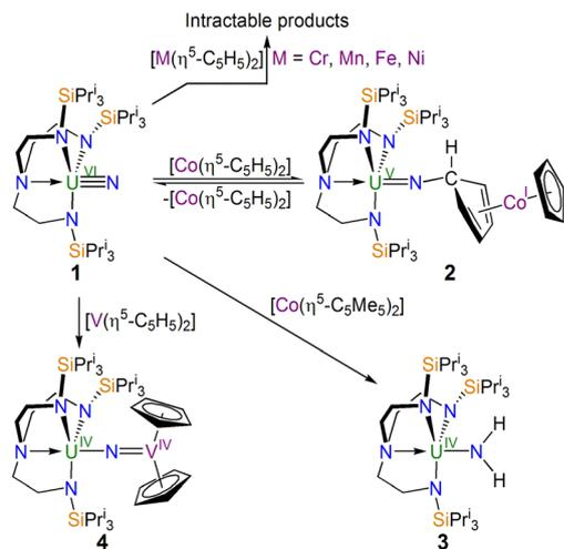
**Scheme 1** Synthesis of **2–4** from **1** and intractable reaction outcomes. The by-products are either not known or are not shown for clarity.
