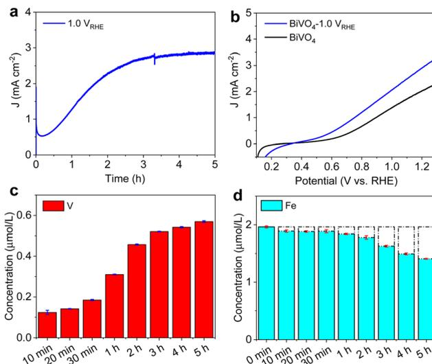
Fig. 2 (a)  $J-t$  curve at 0.6 V vs. RHE of  $\text{BiVO}_4$  photoanodes tested in 1 M KBI pH 9.3 under AM 1.5 G irradiation ( $100 \text{ mW cm}^{-2}$ ). (b) The LSV curves before and after the  $J-t$  curve. ICP results of (c) V and (d) Fe in electrolyte used in the  $J-t$  curve during different times.
