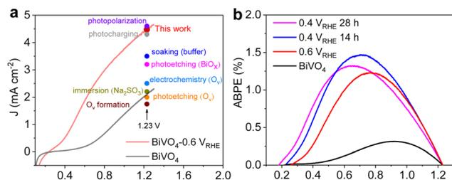
Fig. 5 (a) LSVs of the  $\text{BiVO}_4$  photoanode for the best activation photocurrent in this work, which is also compared with the results of other unmodified  $\text{BiVO}_4$  photoanodes. (b) ABPEs calculated by LSV curves.
