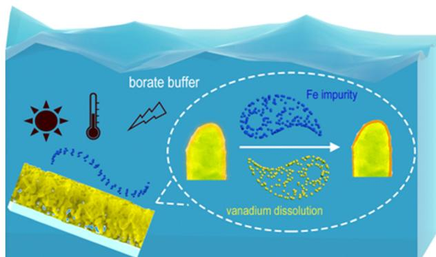
Fig. 1 The borate buffer activation process of the nanoporous  $\text{BiVO}_4$  photoanode, including the formation of an Fe active layer and the dissolution of vanadium species.
