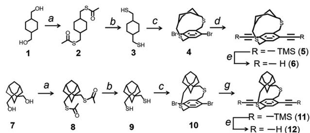
Fig. 5 Synthesis of cycloalkyl strapped monomers. Reaction conditions: (a) thioacetic acid, DIAD, PPh<sub>3</sub>, THF; (b) LiAlH<sub>4</sub>, THF; (c) 2,5-dibromo-*p*-xylylene dibromide, KOH, C<sub>6</sub>H<sub>6</sub>, EtOH; (d) (i) TMS-acetylene, Pd(PPh<sub>3</sub>)<sub>4</sub>, CuI, toluene, triethylamine; (e) TBAF, THF; (g) TMS-acetylene, Pd(PPh<sub>3</sub>)<sub>4</sub>, CuI, piperidine.
