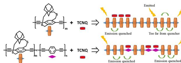
**Fig. 17** Copolymers (bottom) with a mixture of strapped and non-strapped units direct acceptors to strongly interact with the non-strapped units because the  $\pi$ -face is less hindered. The random distribution of non-strapped units increases non-neighbor acceptor binding events and results in higher PL quenching. Reproduced with permission from ref. 53 Copyright American Chemical Society (2023).
