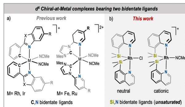
**Fig. 1** Chiral d<sup>6</sup> transition metal complexes: (a) examples of hexacoordinated 18e complexes with two bidentate (CN) ligands and two labile ligands. (b) Pentacoordinated 16e chiral-at-rhodium complexes bearing two bidentate (SiN) ligands developed in this study.
