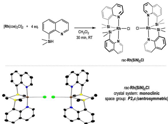
Scheme 1 Synthesis and molecular structure of *rac*-Rh(SiN)<sub>2</sub>Cl complex.<sup>7</sup>
