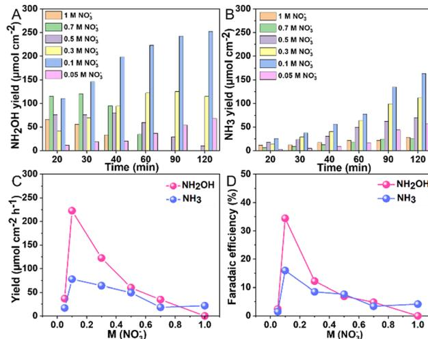
Fig. 3 Variation in  $\text{NH}_2\text{OH}$  (A) and  $\text{NH}_3$  (B) yield rates across different nitrate concentrations at pH 1; performance assessed at an applied potential of  $-0.7$  V vs. RHE over a 2-hour reaction time; (C) yield rates and (D) faradaic efficiency of  $\text{NH}_2\text{OH}$  and  $\text{NH}_3$  across different nitrate concentrations at pH 1 with an applied potential of  $-0.7$  V vs. RHE for a duration of 1 hour.
