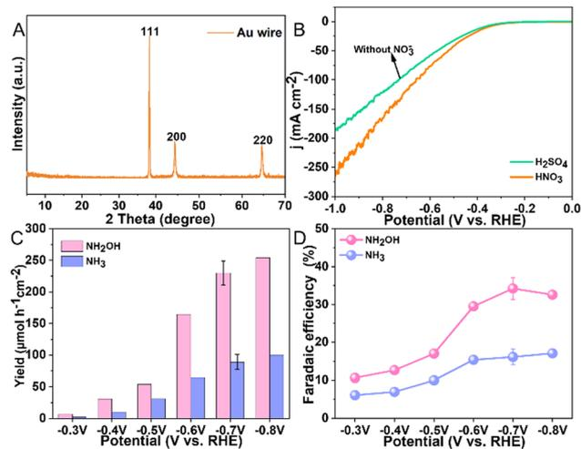
Fig. 2 Characterization and performance of a Au electrode in electrochemical  $\text{NO}_3\text{RR}$ : (A) XRD pattern, (B) comparative LSV curves for the Au wire electrode measured in  $0.1\text{ M HNO}_3$  and  $0.1\text{ M H}_2\text{SO}_4$ , (C) influence of applied potential on the  $\text{NO}_3\text{RR}$  yield rates of  $\text{NH}_2\text{OH}$  and  $\text{NH}_3$ , and (D) faradaic efficiency integrated over 1 hour in  $0.1\text{ M HNO}_3$ .
