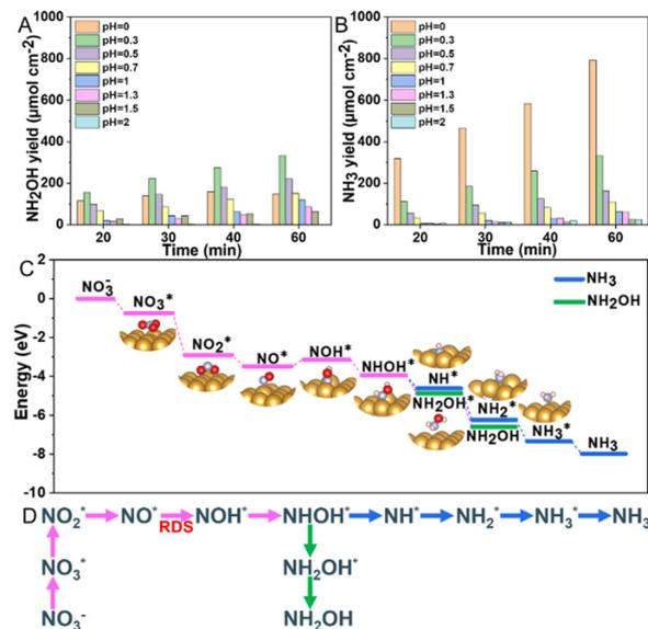
Fig. 4 Yield rates of  $\text{NH}_2\text{OH}$  (A) and  $\text{NH}_3$  (B) across various pH levels, assessed in a solution of 0.1 M  $\text{KNO}_3$  with  $\text{H}_2\text{SO}_4$  adjusting the pH, at an applied potential of  $-0.7$  V vs. RHE for a period of 1 hour; (C) the Gibbs free energy diagram for  $\text{NO}_3\text{RR}$  on Au wire; (D) the possible  $\text{NO}_3\text{RR}$  pathway on the Au electrode.
