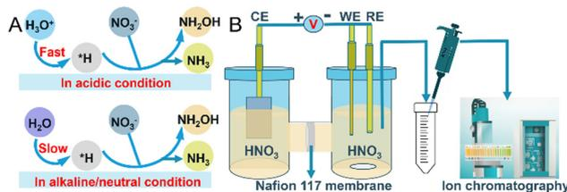
Fig. 1 (A) Pathways for surface adsorbed hydrogen,  $^*H$ , generation under acidic or neutral/alkaline conditions; (B) schematic representation of the experimental approach used for the  $\text{NO}_3\text{RR}$ , including the H-cell configuration and ion chromatography for product analysis.
