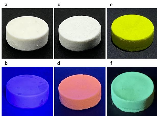
Fig. 2 Photographs of  $(\text{C}_6\text{H}_5\text{-CH}_2\text{-CH}_2\text{-NH}_3)_2\text{PbBr}_4$  (a) and (b),  $(\text{C}_6\text{H}_5\text{-CH}_2\text{-CH}_2\text{-NH}_3)_2\text{Pb}_{0.977}\text{Mn}_{0.023}\text{Br}_4$  (c) and (d), and  $(\text{C}_6\text{H}_5\text{-CH}_2\text{-CH}_2\text{-NH}_3)_2\text{PbBr}_3\text{I}$  (e) and (f) aerogels under white (a), (c) and (e) and 365-nm ultraviolet light (b), (d) and (f). Diameters of the aerogels were 16 mm.
