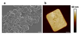
Fig. 1 SEM (a) and AFM (b) images of  $(C_6H_5-CH_2-CH_2-NH_3)_2PbBr_4$ nanoplatelets. Scale bars: (a) 1 μm, (b) 200 nm.
