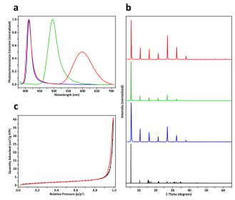
Fig. 3 (a) and (b) Emission spectra (a) and PXRD patterns (b) of  $(C_6H_5-$ CH2-CH2-NH3)2PbBr4 (blue; simulated PXRD profile depicted in black),  $(C_6H_5-CH_2-CH_2-NH_3)_2PbBr_3I_1$  (green), and  $(C_6H_5-CH_2-CH_2-NH_3)_2-RH_3$ Pb<sub>0.977</sub>Mn<sub>0.023</sub>Br<sub>4</sub> (red) aerogels. (c) Nitrogen adsorption-desorption isotherms of  $(C_6H_5-CH_2-CH_2-NH_3)_2PbBr_4$  aerogels.
