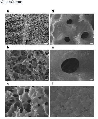
Fig. 4 Cross-sectional SEM images of a (C<sub>6</sub>H<sub>5</sub>-CH<sub>2</sub>-CH<sub>2</sub>-NH<sub>3</sub>)<sub>2</sub>PbBr<sub>4</sub> aerogel. Scale bars: (a) 200  $\mu$ m, (b) 50  $\mu$ m, (c) 20  $\mu$ m, (d) 10  $\mu$ m, (e) 4  $\mu$ m, (f) 500 nm
