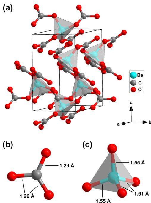
Fig. 3 (a) Trigonal crystal structure ( $P3_121$ ,  $Z = 3$ ) of Be(CO<sub>3</sub>) at 20(2) GPa obtained from synchrotron X-ray single crystal structure solution. (b) Geometry of the [CO<sub>3</sub>]<sup>2-</sup>-groups and (c) of the BeO<sub>4</sub>-tetrahedra in Be(CO<sub>3</sub>).
