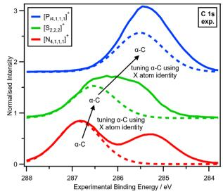
Fig. 4 Tuning  $\alpha$ -C using X atom identity. Experimental C 1s XP spectra for  $[P_{i4,1,1,1}][NTf_2]$ ,  $[S_{2,2,2}][NTf_2]$  and  $[N_{4,1,1,1}][NTf_2]$  ionic liquids. Experimental XP spectra are area normalised and charge referenced using methods given in ESI,† Section S5. Traces are vertically offset for clarity.
