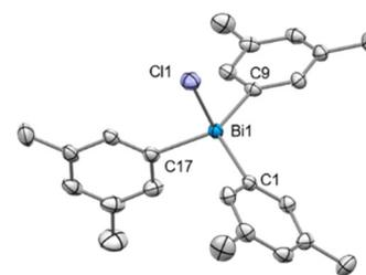
Fig. 3 Solid state structure of **10**. Ellipsoids are drawn at the 50% probability level. H atoms and  $\text{BAR}^{\text{F}}$  are omitted for clarity. Selected bond lengths (Å) and angles ( $^\circ$ ): Bi1–Cl1: 2.4028(8), Bi1–C1: 2.185(3), Bi1–C9: 2.180(3), Bi1–C17: 2.189(3), C1–Bi1–C9: 121.63(11), C1–Bi2–C17: 111.32(10), C9–Bi2–C17: 112.55(11).
