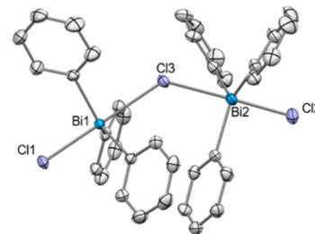
Fig. 2 Solid state structure of **9a**.<sup>29</sup> Ellipsoids are drawn at the 50% probability level. H atoms, disordered parts and  $\text{BAR}^{\text{F}}$  are omitted for clarity. Selected bond lengths (Å) and angles ( $^\circ$ ): Bi1–Cl1: 2.4856(7), Bi1–Cl3: 2.7995(7), Bi2–Cl2: 2.4996(8), Bi2–Cl3: 2.8274(7), Bi1–Cl3–Bi2: 128.10(2); Cl1–Bi1–Cl3: 179.25(2), Cl2–Bi2–Cl3: 177.70(2).
