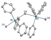
Fig. 2 Solid state structure of **9a**.<sup>29</sup> Ellipsoids are drawn at the 50% probability level. H atoms, disordered parts and BArF are omitted for clarity. Selected bond lengths (Å) and angles (°): Bi1-Cl1: 2.4856(7), Bi1-Cl3: 2.7995(7), Bi2-Cl2: 2.4996(8), Bi2-Cl3: 2.8274(7), Bi1-Cl3-Bi2: 128.10(2); Cl1-Bi1-Cl3: 179.25(2), Cl2-Bi2-Cl3: 177.70(2).
