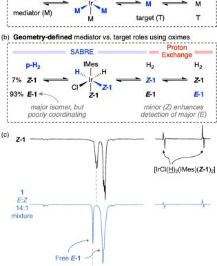
Fig. 3 (a) Typical roles of mediator and target in SABRE-relay, with (b) geometric isomers of oximes playing different roles. (c) Hyperpolarised <sup>1</sup>H NMR spectra of a mixture of E and Z isomers of oxime **1**.
