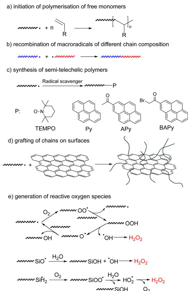
**Fig. 3** Five types of synthetic applications of mechanochemically-generated macroradicals: (a–c) homogeneous formation of new backbone bonds; (d) interphasial bond formation; (e) chemistries mediated by small molecules. Wavy lines represent polymer chains.
