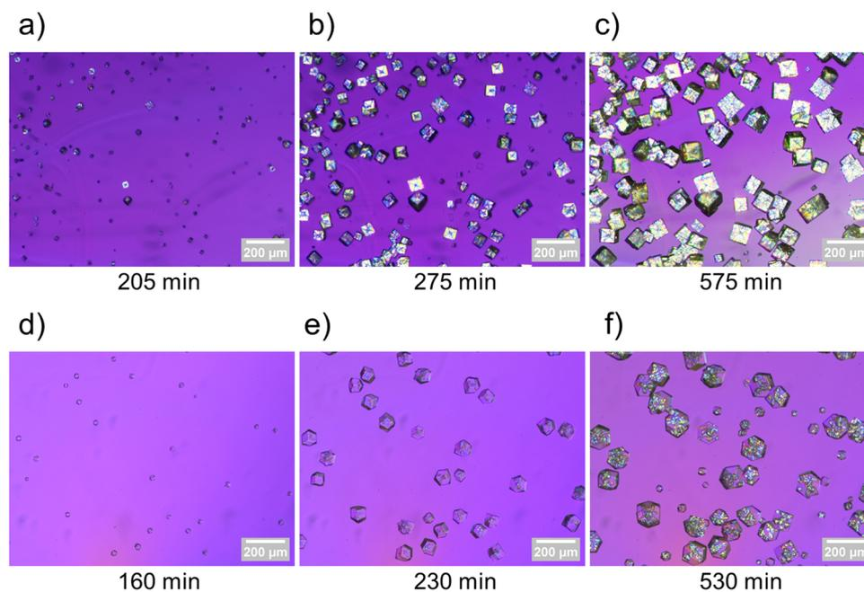
**Fig. 2** Images of IRMOF-9 crystals at 205 min (a), 275 min (b), and 575 min (c) into synthesis. Images of IRMOF-9/10 crystals at 160 min (d), 230 min (e), and 530 min (f) into synthesis.
