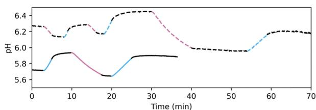
Fig. 5 A solution of **PBD2** (0.40 mM) and **PAD3** (0.63 mM) in 50% methanol in water was alternately irradiated with 450 nm (pink) and 310 nm (blue) light. A black line indicates no irradiation. The initial pH (6.05) was adjusted by the addition of small amounts of acetic acid and triethylamine.
