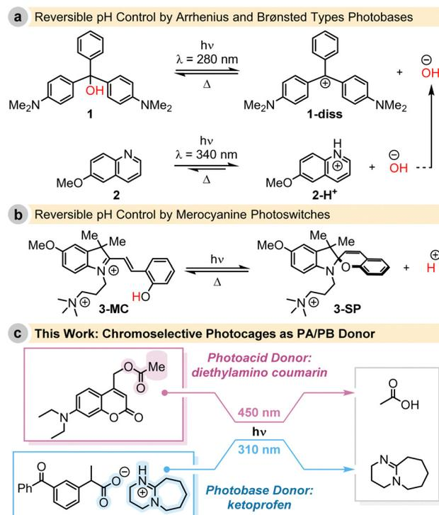
**Fig. 1** (a) Reversible pH control by Arrhenius and Brønsted types photobase generator; (b) reversible pH control by Merocyanine photoswitches; (c) our approach: chromoselective pH regulation by photocages as photoacid/photobase donors.
