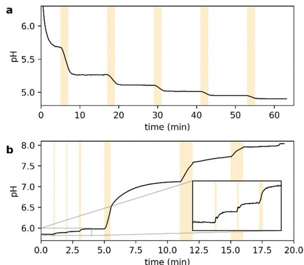
Fig. 4 (a) A saturated solution of **PAD3** (<2 mM) in 50% methanol in water is irradiated 5 times with 365 nm light for 120 s, as indicated by the yellow shading, while simultaneously the pH is measured. (b) A solution of **PBD2** (2.5 mM) in 50% methanol in water is irradiated with 365 nm light for 5, 5, 10, 30, 60, and 60 s.
