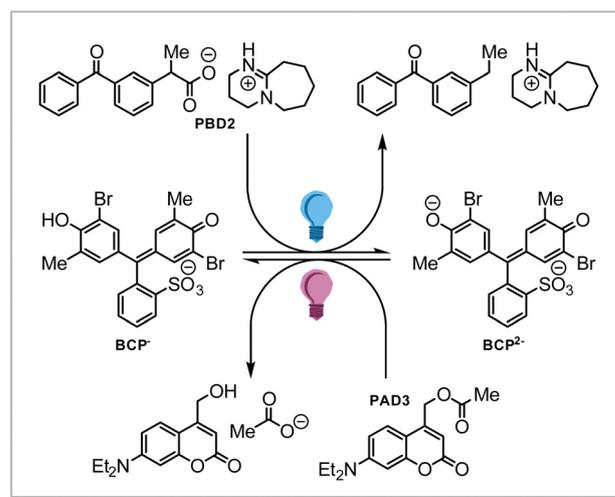
Scheme 2 Change in protonation state of bromocresol purple (**BCP**) from **BCP<sup>-</sup>** to **BCP<sup>2-</sup>**.
