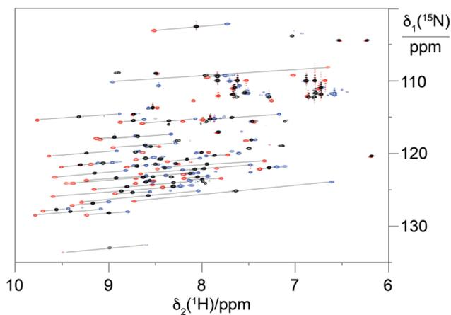
Fig. 3 Superimposition of  $^{15}\text{N}$ -HSQC spectra of ubiquitin S57C ligated with the **C14** tag loaded with different metal ions. The spectra recorded with diamagnetic **Y.C14** tag and paramagnetic **Tm.C14** and **Tb.C14** are plotted in black, blue and red, respectively. Lines link paramagnetic with diamagnetic cross-peaks, identifying the PCSs.
