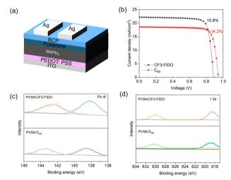
Fig. 3 Device performance and evaluations. (a) Schematic diagram of device structure. (b) J-V curve of the device with the best PCE. (c) and (d) XPS experiment plot and fitting curve of the Pb 4f orbital and I 3d orbital.
