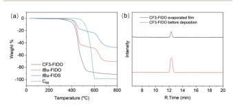
Fig. 1 Thermal stability of fullerene derivatives. (a) Vacuum TGA. (b) HPLC chart before and after evaporation of CF3-FIDO
