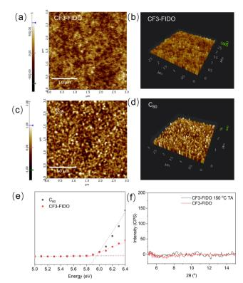
Fig. 2 Film characterization of evaporated film. (a) – (d) AFM of evaporated film. (e) PYS of fullerenes. (f) GIXRD of CF3-FIDO film for different annealing temperatures.
