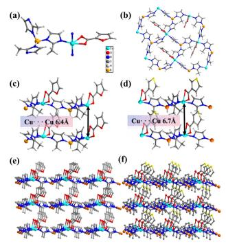
Fig. 1 (a) Coordination environment of BIF-151; (b) the 2D layer structure of BIF-151; the Cu···Cu distance between adjacent lawyer of (c) BIF-151 and (d) BIF-154; the 3D stacking model of (e) BIF-151 and (f) BIF-154.
