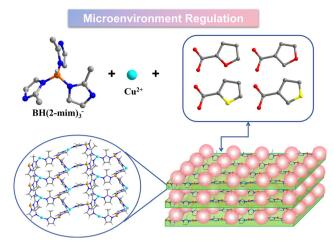
Scheme 1 Synthesis procedure and the layer structure diagram. The pink sphere denotes the second ligand and the light green lamellar represents CuBH(mim)<sub>3</sub>+ layer.
