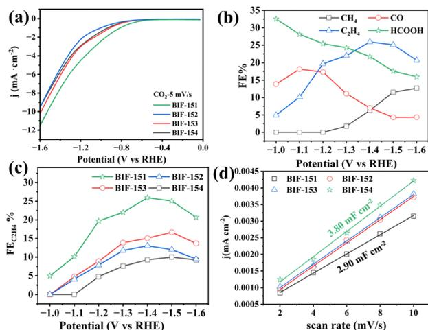
Fig. 3 (a) LSV curves of BIF-151, BIF-152, BIF-153 and BIF-154 electrocatalysts in CO<sub>2</sub> saturated 0.5 M KHCO<sub>3</sub> electrolyte, respectively; (b) the FE of gas products and liquid products of BIF-151 electrocatalyst at different applied potentials in CO<sub>2</sub> saturated electrolyte; (c) the FE<sub>C<sub>2</sub>H<sub>4</sub></sub> of BIF-151, BIF-152, BIF-153, and BIF-154 electrocatalyst; (d) the C<sub>dl</sub> of BIF-151, BIF-152, BIF-153, and BIF-154 electrocatalyst.
