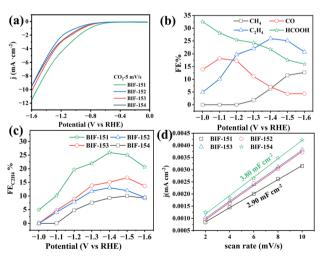
Fig. 3 (a) LSV curves of BIF-151, BIF-152, BIF-153 and BIF-154 electrocatalysts in CO<sub>2</sub> saturated 0.5 M KHCO<sub>3</sub> electrolyte, respectively; (b) the FE of gas products and liquid products of BIF-151 electrocatalyst at different applied potentials in  $CO_2$  saturated electrolyte; (c) the  $FE_{C_2H_4}$  of BIF-151, BIF-152, BIF-153, and BIF-154 electrocatalyst; (d) the  $C_{\rm dl}$  of BIF-151, BIF-152, BIF-153, and BIF-154 electrocatalyst.
