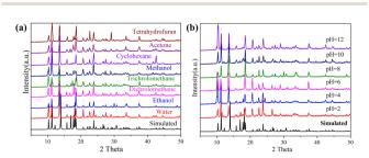
Fig. 2 The powder XRD patterns of BIF-151: (a) solvent stability and (b) chemical stability
