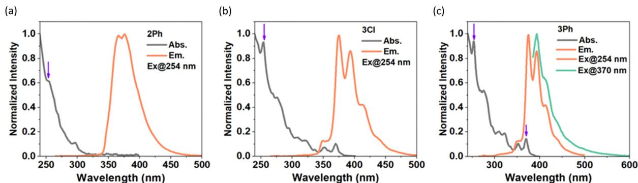
Fig. 3 Absorption and emission spectra of (a) **2Ph**, (b) **3Cl**, and (c) **3Ph** in CH<sub>2</sub>Cl<sub>2</sub> ( $< 10^{-5}$  M). The linear dependence of absorbance on concentration is presented in Fig. S23 (ESI<sup>†</sup>), and excitation spectra are provided in Fig. S24 (ESI<sup>†</sup>).
