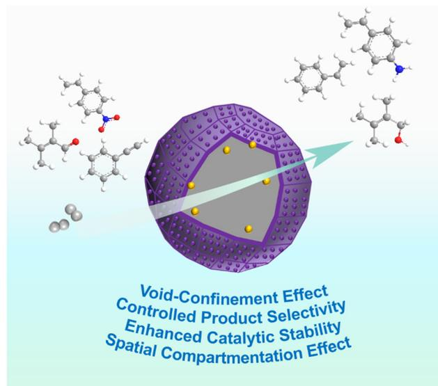
Fig. 4 Schematic illustration of the properties of HSNRs applied in liquid-phase hydrogenation reactions.
