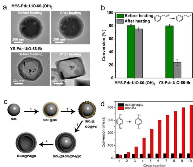
Fig. 7 (a) TEM images of HSNRs with different nanostructures before and after heating; (b) catalytic conversion of allylbenzene on HSNRs.<sup>49</sup> Copyright 2019, American Chemical Society. (c) Schematics of the synthesis of RGO@Pd@C hollow spheres; (d) the stability testing of these nanocatalysts.<sup>72</sup> Copyright 2014, Nature Publishing Group.
