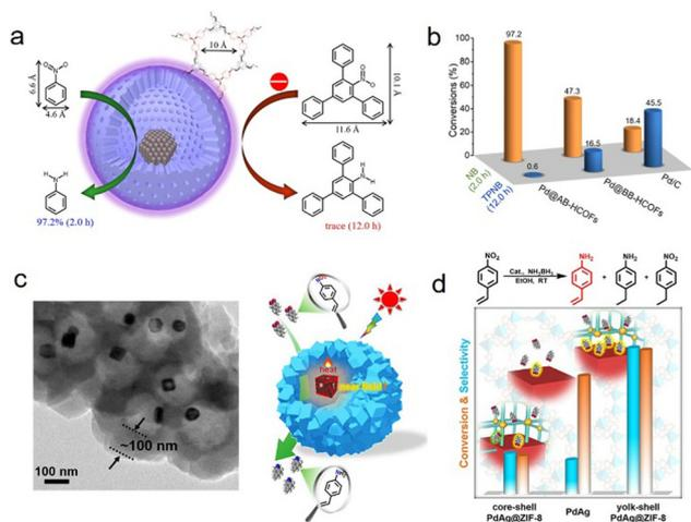
Fig. 6 (a) Schematic illustration for the size-selectivity of a Pd@AB-HCOFs nanoreactor in nitroarene hydrogenation; (b) catalytic activity comparisons of various catalysts.<sup>65</sup> Copyright 2022, American Chemical Society. (c) TEM image and structural model of a core-shell PdAg@ZIF-8 nanoreactor; (d) chemoselective hydrogenation of nitrostyrene with different catalysts.<sup>67</sup> Copyright 2022, American Chemical Society.
