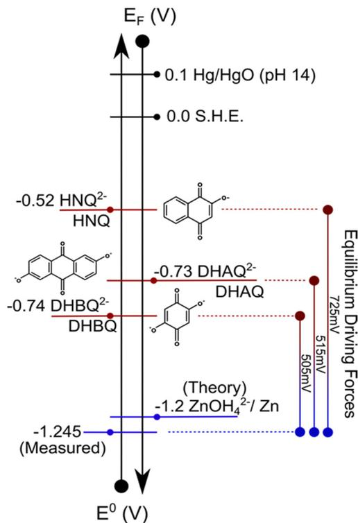
Fig. 1 Electrode potential scale showing the location of the approximate redox potentials both *versus* a standard reference ( $E^0$ ) and absolute electron energy ( $E_F$ ), for both the zinc/zincate couple and quinone redox couples selected as mediators. Equilibrium overpotentials between the liquid/solid components are indicated on the right-hand side. Please see ESI† for complete compound names and discussion of reactions.
