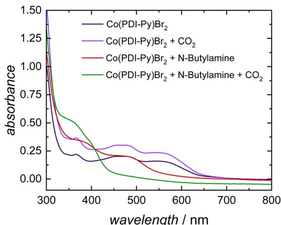
Fig. 3 Absorption measurements of 0.1 mM  $[\text{Co}(\text{PDI-Py})\text{Br}_2]$  in MeCN solutions containing 0.03 M  $n\text{Bu}_4\text{NPF}_6$  and 11 M  $\text{H}_2\text{O}$  in  $\text{N}_2$ -sparged solution (blue line),  $\text{CO}_2$ -saturated solution (purple line),  $\text{N}_2$ -sparged solution with 6.6 mM NBA (red line), and  $\text{CO}_2$ -saturated solution with 6.6 mM NBA (green line).
