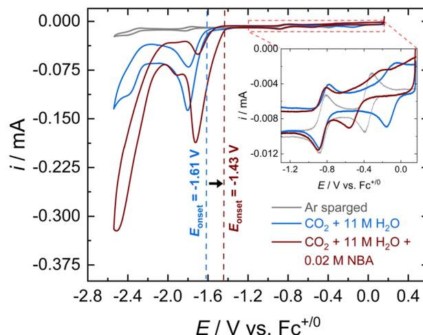
Fig. 1 Representative CVs of 0.3 mM [Co(PDI-Py)] in MeCN with 0.1 M *n*Bu<sub>4</sub>NPF<sub>6</sub> at a scan rate of 0.05 V s<sup>-1</sup>. CVs were taken in Ar-sparged solution (gray line), CO<sub>2</sub>-saturated solution containing 11 M H<sub>2</sub>O (red line), and CO<sub>2</sub>-saturated solution containing 11 M H<sub>2</sub>O and 0.2 M NBA (blue line). The inset is a zoom in of the region in the dashed orange box showing the Co<sup>3+/2+</sup> and Co<sup>2+/+</sup> peaks.
