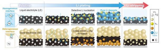
Schematic illustration showing the comparative alloying reactions of Ag/C with Li in LE and SE.
