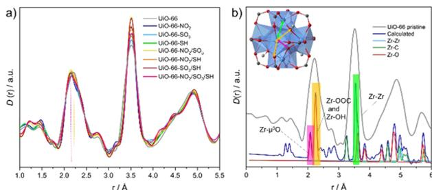
**Fig. 2** (a) PDF of the MOFs in the 1.0–5.5 Å range showing peaks centred at 2.2 and 3.5 Å typical from Zr–O and Zr···Zr correlations, respectively. (b) Comparison of the experimental  $D(r)$  of the pristine UiO-66 with the calculated partial  $g(r)$ s using PDFGUI (ADP values are approached to 0.0005). Main correlations are highlighted in pink, yellow and green.
