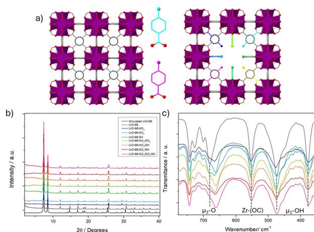
Fig. 1 (a) Schematic representation of MTVM MOF with defect-induced *reo* topology compared with the pristine MOF. (b) PXRD profiles (c) FT-IR profiles highlighting  $\mu_3$ -O,  $\mu_3$ -OH and Zr-(OC) bands.
