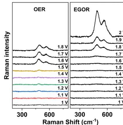
Fig. 5 Potential-dependent Raman spectra of a Ni foam anode in the absence of ethylene glycol (left, OER) and in the presence of ethylene glycol (EGOR, right).
