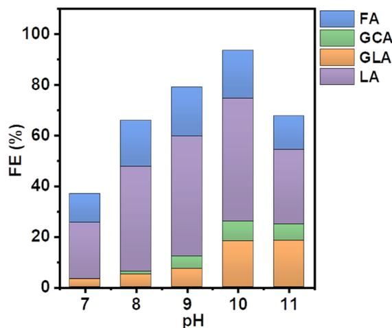
Fig. 3 Faraday efficiencies (FE) of the EGOR at a constant current density of  $5 \text{ mA cm}^{-2}$  at various pH conditions in the presence of borate.
