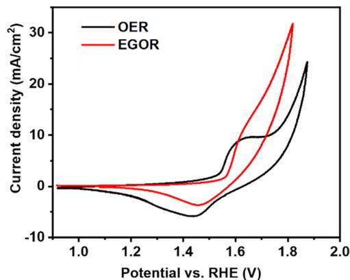
Fig. 1 CV at a Ni foam electrode in the absence and presence of 0.1 M ethylene glycol in borate buffer solution at pH 10 at a scan rate of  $10 \text{ mV s}^{-1}$ .
