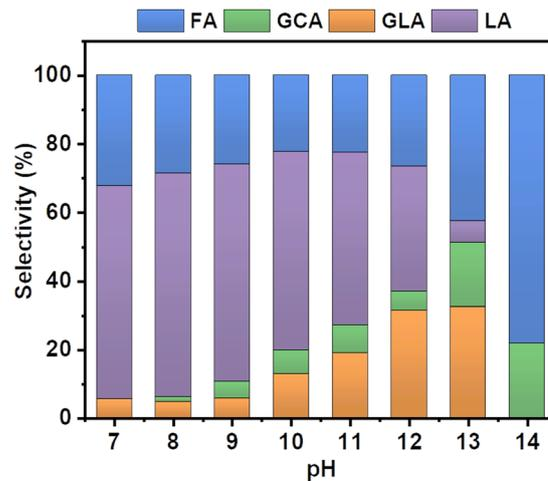
Fig. 2 Product selectivity of the EGOR after one hour of electrolysis at a constant current density of  $5 \text{ mA cm}^{-2}$  at various pH conditions. Formic acid (FA), lactic acid (LA), glycolic acid (GCA), and glyceric acid (GLA).
