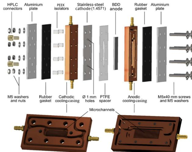
Fig. 4 Custom-developed electrolyser based on copper-based cooling cell.<sup>45</sup> Copyright (2023) Wiley. Used with permission from Seitz *et al.* Concentrated aqueous peroxodicarbonate: efficient electro-synthesis and use as an oxidizer in epoxidations, S- and N-oxidations, *Angew. Chem. Int. Ed.*, Wiley.
