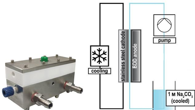
Fig. 2 Flow electrolyser developed by Zirbes *et al.*<sup>48</sup> Copyright (2023) Wiley. Used with permission from Zirbes *et al.* Peroxodicarbonate as a green oxidizer for the selective degradation of kraft lignin into vanillin, *Angew. Chem. Int. Ed.*, Wiley.
