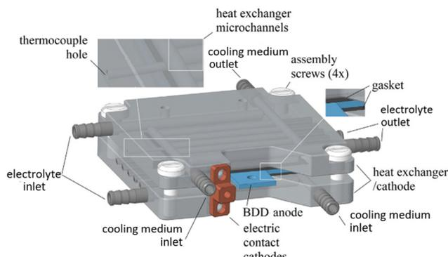
Fig. 3 CAD image of the ECMR assembly.<sup>44</sup> Copyright (2023) Elsevier. Used with permission from Ziogas *et al.* Peroxodicarbonate: Electro-synthesis and first directions to green industrial applications, *Curr. Res. Green Sustainable Chem.*, Elsevier.
