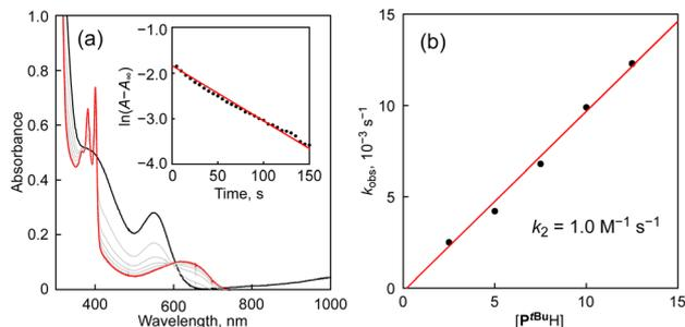
Fig. 2 (a) UV-vis spectral changes for the reaction of  $1^{\text{Br}}$  (0.25 mM) with 2,4,6-tri-*tert*-butylphenol ( $\text{P}^{\text{tBuH}}$ , 12.5 mM) in  $\text{CH}_3\text{CN}$  at  $0^\circ\text{C}$ . Inset: A pseudo-first-order plot based on the absorption change at 410 nm. (b) Plot of  $k_{\text{obs}}$  vs. substrate concentration.
