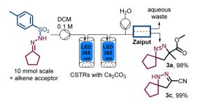
Scheme 4 Photo-CSTR cascade with integrated in-line work up using Zaiput membrane technology. Reaction conditions: N-tosylhydrazone 1a, 1c (15 or 12 mmol), acrylate 2a (10 mmol), Cs<sub>2</sub>CO<sub>3</sub> (15 or 12 mmol), DCM 0.1 M (100 mL), CSTR ( $\lambda$  = 365 nm, 36.7 W or 50 W, 500 rpm), 35 °C, 20 or 30 min. Typical run 2 h ( $t_{Res}$  116 min) incl. flushing CSTR with DCM.
