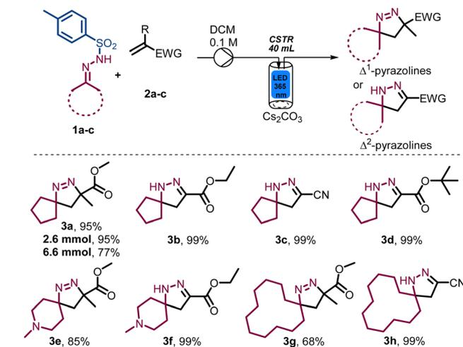
Scheme 2 Reaction scope towards spirocyclic  $\Delta^1$ -pyrazolines and  $\Delta^2$ -pyrazolines. Reaction conditions: *N*-tosylhydrazone **1a-c** (2.4 or 3 mmol), acrylate **2a-c** (2 mmol),  $\text{Cs}_2\text{CO}_3$  (2.4 or 3 mmol), DCM 0.1 M (20 mL), CSTR ( $\lambda = 365$  nm, 36.7 W or 50 W, 500 rpm), 35 °C, 20 or 30 min.
