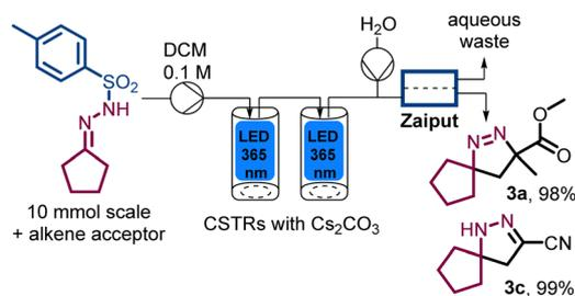
**Scheme 4** Photo-CSTR cascade with integrated in-line work up using Zaiput membrane technology. Reaction conditions: *N*-tosylhydrazone **1a**, **1c** (15 or 12 mmol), acrylate **2a** (10 mmol),  $\text{Cs}_2\text{CO}_3$  (15 or 12 mmol), DCM 0.1 M (100 mL), CSTR ( $\lambda = 365$  nm, 36.7 W or 50 W, 500 rpm), 35 °C, 20 or 30 min. Typical run 2 h ( $t_{\text{res}}$  116 min) incl. flushing CSTR with DCM.
