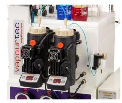
Fig. 1 Image of photo-CSTR module with Vapourtec E-Series flow
