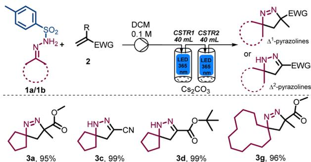
**Scheme 3** Improved reaction performance and scale-up using two sequential photo-CSTRs. Reaction conditions: *N*-tosylhydrazone **1a**, **1b** (15 or 12 mmol), acrylate **2a**, **2c** (10 mmol),  $\text{Cs}_2\text{CO}_3$  (15 or 12 mmol), DCM 0.1 M (20 mL), CSTR ( $\lambda = 365$  nm, 36.7 W or 50 W, 500 rpm), 35 °C, 20 or 30 min.
