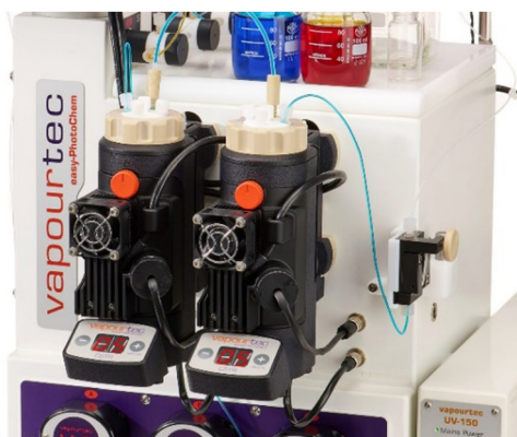
Fig. 1 Image of photo-CSTR module with Vapourtec E-Series flow reactor.
