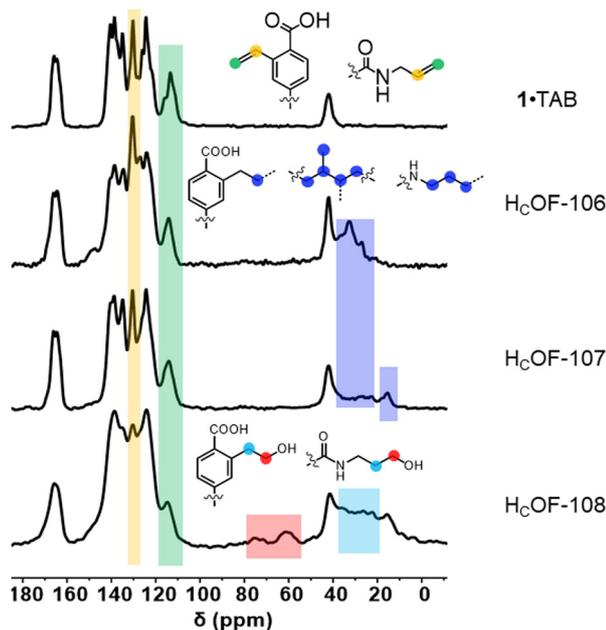
Fig. 2 Stacked solid-state  $^{13}\text{C}$  NMR spectra of **1**-TAB,  $\text{H}_\text{C}\text{OF-106}$ ,  $\text{H}_\text{C}\text{OF-107}$ , and  $\text{H}_\text{C}\text{OF-108}$  from top to bottom, respectively.
