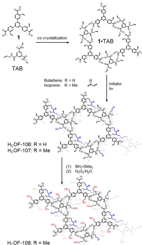
**Scheme 1** Synthesis of H<sub>c</sub>OF-106 and H<sub>c</sub>OF-107 through free-radical reactions with butadiene and isoprene. Post-modification of the single-crystalline H<sub>c</sub>OF-107 affords its hydroxylated derivative H<sub>c</sub>OF-108.
