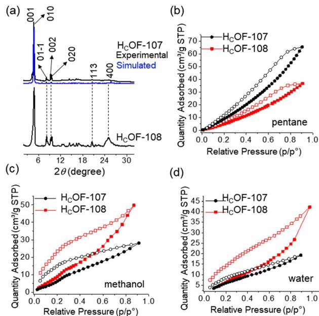
Fig. 4 (a) Simulated (H<sub>C</sub>OF-107) and experimental PXRD patterns of H<sub>C</sub>OF-107 and H<sub>C</sub>OF-108. (b) Pentane, (c) methanol, and (d) water vapor sorption isotherms (295 K) for H<sub>C</sub>OF-107 (black) and H<sub>C</sub>OF-108 (red).
