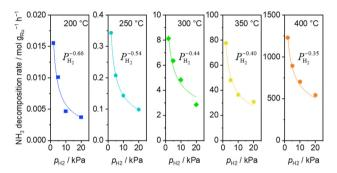
Fig. 3 H<sub>2</sub> pressure dependence of ammonia decomposition rates over 0.1 mg of 5 wt% Ru/CeO<sub>2</sub> diluted with 9.9 mg of CeO<sub>2</sub> within the pellets at 200 (blue square), 250 (light blue circle) and 300 °C (green diamond) and over 1 mg pellets of  $10\times$  further dilution with CeO<sub>2</sub> within pellets at 350 (yellow pentagon) and 400 °C (orange pentagon) (5 kPa NH<sub>3</sub>, balanced by Ar). Raw data are shown in Fig. S5 (ESI†).
