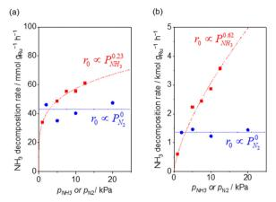
**Fig. 2** NH<sub>3</sub> (red square) and N<sub>2</sub> (blue circle) pressure dependence of ammonia decomposition rates (a) over 0.1 mg of 5 wt% Ru/CeO<sub>2</sub> diluted with 9.9 mg of CeO<sub>2</sub> within pellets at 200 °C and (b) over 1 mg pellets of  $10\times$  further dilution with CeO<sub>2</sub> within the pellets at 400 °C. Initial conditions:  $\sim$  0.5 kPa NH<sub>3</sub> balanced with Ar, total 101 kPa. Raw data are shown in Fig. S3 and S4 (ESI†).
