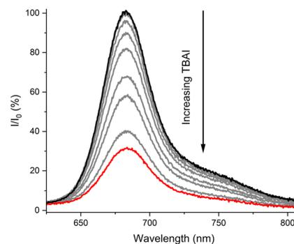
Fig. 3 Normalised fluorescence emission response of 1  $\mu$ M sensor **1** upon addition of increasing concentrations of I<sup>-</sup> (up to 2.8 mM) in acetone at 298 K.
