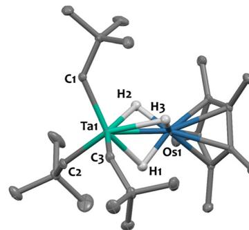
Fig. 1 Solid-state molecular structure of **2** (30% probability ellipsoids). Hydrogen atoms from the hydrocarbon ligands are omitted for clarity. Selected bond distances (Å) and angles (°): Ta1–Os1 2.4817(2), Ta1–C1 2.132(3), Ta1–C2 2.136(3), Ta1–C3 2.143(3), Os1–H1 1.45(5), Os1–H2 1.56(5), Os1–H3 1.48(8), Ta1–H1 2.07(5), Ta1–H2 2.03(5), Ta1–H3 2.07(8), Ta1–Os1– $\text{Cp}^*\text{centroid}$  178.1(1).
