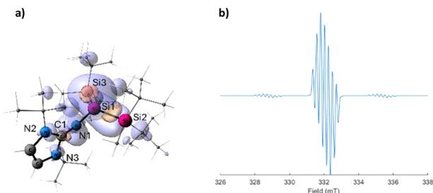
**Fig. 3** (a) Optimized structure of **2** (iso = 0.04) and the calculated spin density map (purple – positive, orange – negative), at the B3LYP/IGLO-III//r<sup>2</sup>SCAN-3c level of theory. Mulliken spin populations of selected atoms: Si1 (0.922), Si2 (−0.040), Si3 (−0.030), N1 (0.106), N2 (0.009), N3 (0.004). (b) Simulated EPR spectrum using the computationally obtained EPR values (Table 1).
