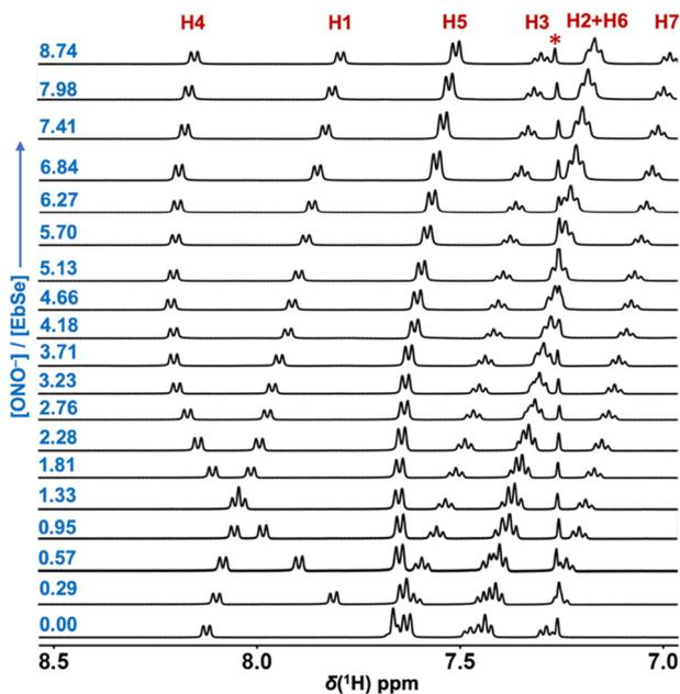
Fig. 4  $^1\text{H}$  NMR spectra of **EbSe** in  $\text{CDCl}_3$  at room temperature upon increasing the ratio of nitrite anion and **EbSe** from 0.00 to 8.74 (as shown in the left panel). The peak marked with \* originates from the  $\text{CDCl}_3$  solvent residual peak. See Fig. 2A for the numbering scheme.
