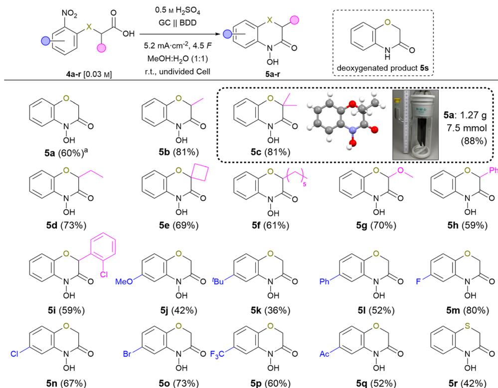
Scheme 3 Scope of the electrochemical synthesis of 2H,4H-4-hydroxy-1,4-benzoxazin-3-ones, isolated yields. <sup>a</sup>Temperature: 10 °C.
