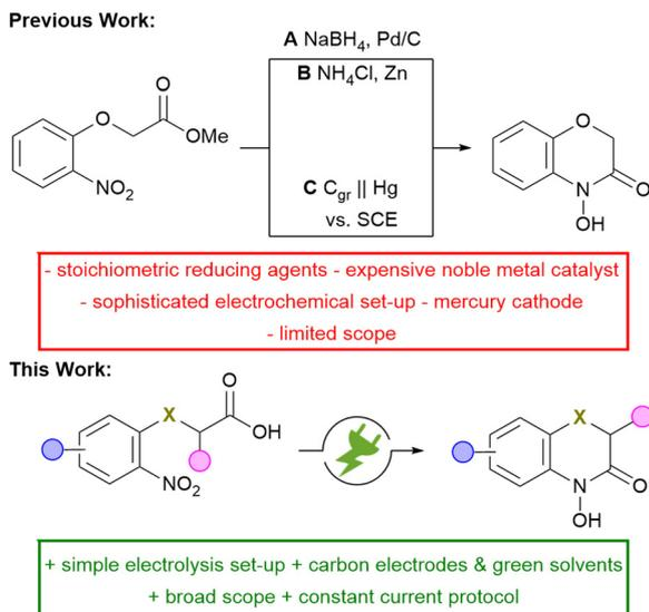
**Scheme 2** Conventional and electrochemical reduction of nitroarenes for the synthesis of 2H,4H-4-hydroxy-1,4-benzoxazin-3-ones; C<sub>gr</sub> = graphite.
