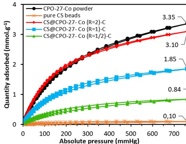
Fig. 3 CO<sub>2</sub> adsorption isotherms of the as-synthesized CPO-27-Co powder, pure CS beads, and CS@CPO-27-Co (*R*) beads measured at 298 K.
