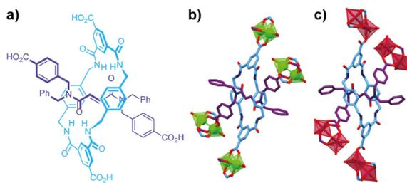
**Fig. 1** (a) Chemical structure of the tetratopic rotaxane ligand **1**. Stick representation of a single unit of the rotaxane ligand coordinated to (b) four Cu(II) paddlewheel clusters of **UMUMOF-7** and (c) four Co(II) clusters of **UMUMOF-8**. Metals are shown in polyhedral representation (colored in green for copper and red for cobalt) and hydrogens are omitted.
