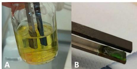
**Fig. 1** (A) Solution of **3** in MeCN/H<sub>2</sub>O with PPh<sub>4</sub>Br electrolyte in Asynt ElectroReact<sup>®</sup> following electrolysis at a fixed potential; (B) the graphite and SS electrodes after Ni recovery. Note the green film deposits on the SS electrode.
