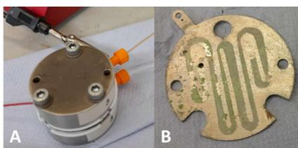
**Fig. 3** (A) Assembled electrochemical flow cell in operation; (B) SS electrode after electrochemical recovery of **3** in MeCN/H<sub>2</sub>O.
